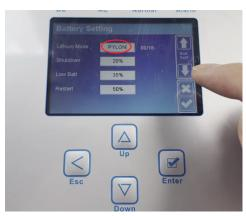
Inverter battery mode select *Lithium*, Lithium type select *PYLON*.
